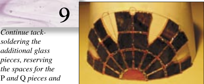
Beginning with the bottom row of glass, place the glass pieces on the form and tack-solder them together.
