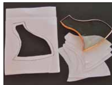
Using copy paper to lift the bevels to the same visual plane as the surrounding glass
