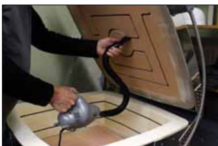
Vacuuming kiln element grooves
