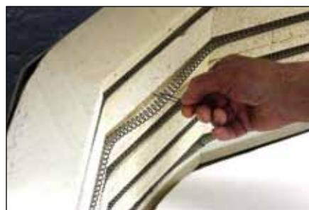
Inserting a new element pin
