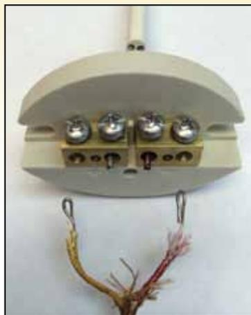
*Note that one of the thermocouple wires is marked red. That is the side that should attract a magnet. If you think the wire may have been incorrectly marked red, touch the wire to the door magnet on a bead kiln or a magnetized screwdriver tip to check it.*
