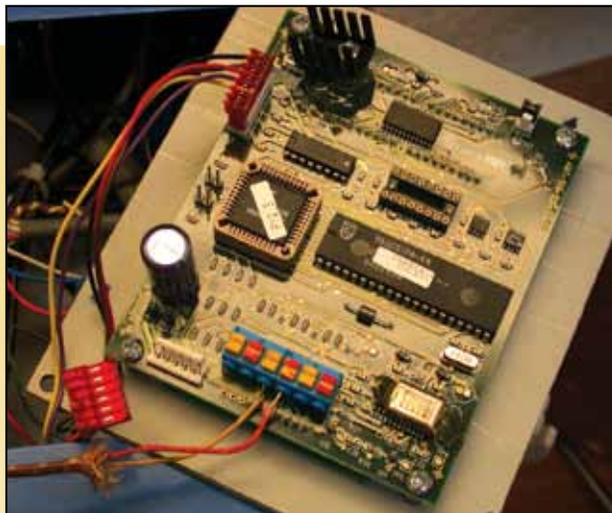
*When reinstalling the controller, avoid twisting the thermocouple wires, which can cause them to touch at the bare ends. This will give a low reading.*
