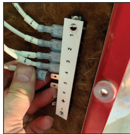
(Photo 3) Since the power strip shown here is near the insulation, you must be careful to keep the insulation out of the wire connectors. The first rule of kilns is that electrical connections must be tight and clean.
