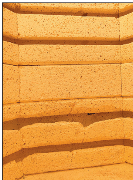
(Photo 2) Compare the bottom element grooves with the ones above. Notice how the bottom grooves have rounded edges and missing firebrick chunks. To avoid this, first remove the element pins, which are not always easy to find. Then roll the element out of the groove the same way you would roll a pencil in your fingers.
