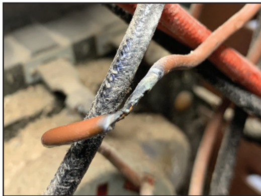
(Photo 1) The insulation on the white wire was burned by contact with an element connector.
