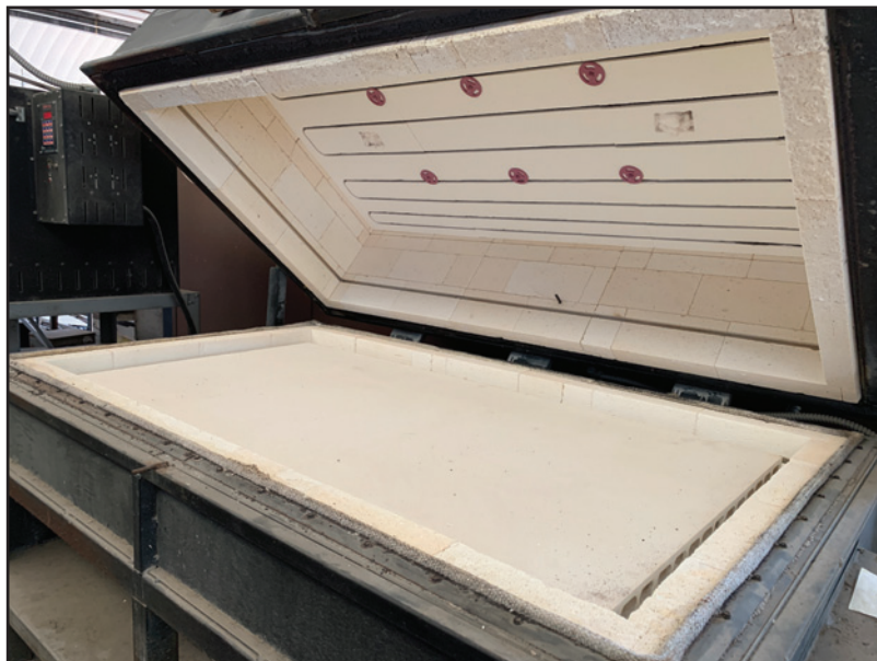
The massive Paragon Pearl-56 has elements in the top, four sides, and bottom, so it fires differently than a kiln with elements only in the top or sides.
