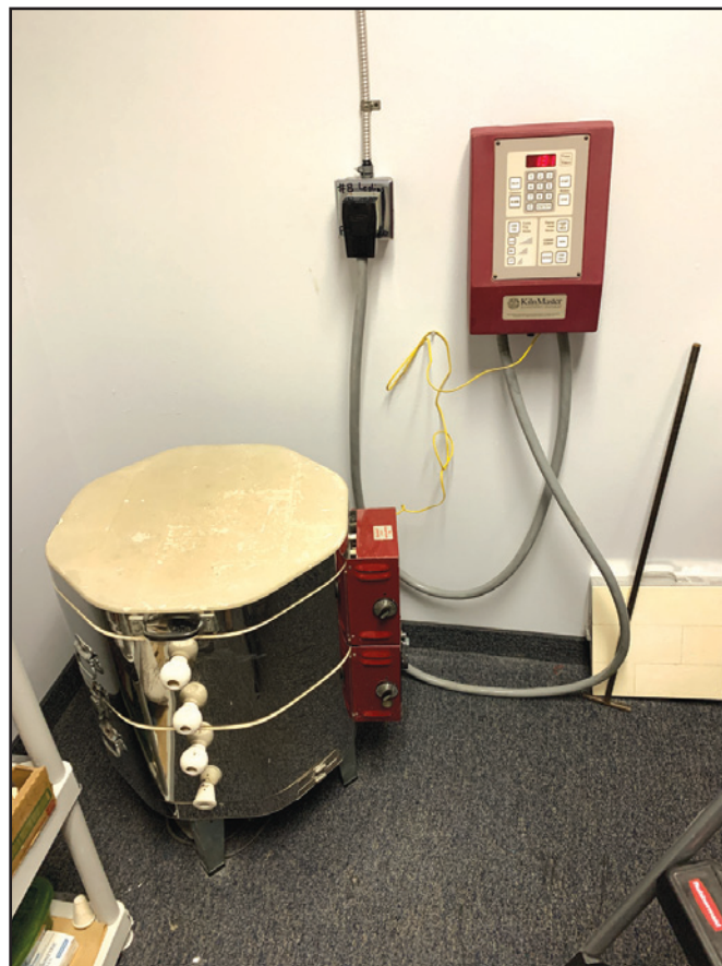
In the Skutt ceramic kiln, with elements only in the walls, glass must be fired slowly, which is why a normal glass firing schedule may need to be altered for this kiln.
