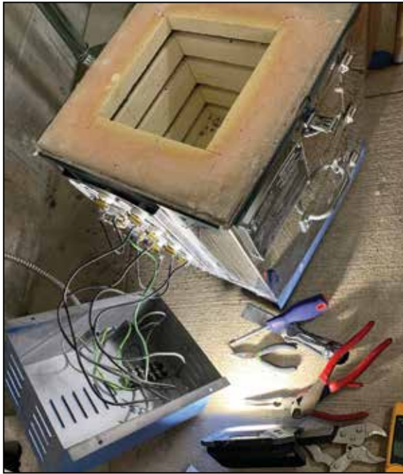
This 240 volt crucible kiln was rated to 2350°F, but it couldn't fire hotter than 2000°F because it was plugged into a 208 volt circuit.
