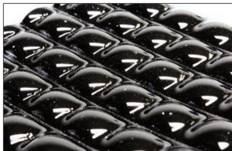
Bumps created firing to 1350°F
