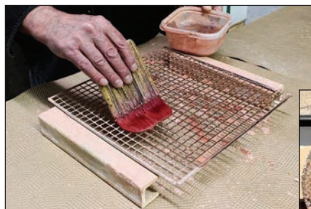
1 Apply 4 coats of kiln wash to the screen.
