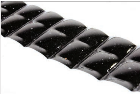
Bumps created firing to 1300°F
