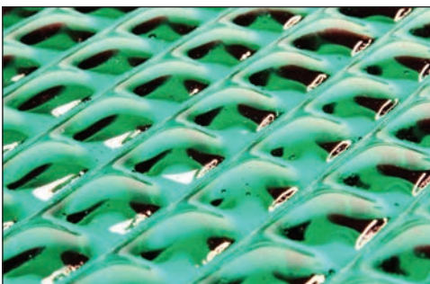
Bumps created firing to 1325°F
